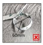
Do not bend XLT tape to a diameter less than 60mm (2.36 inches).
